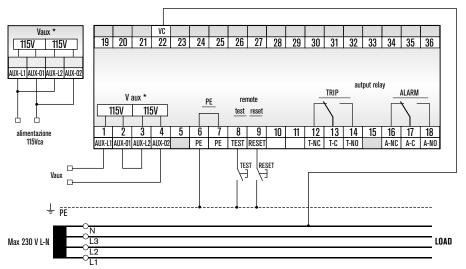
$^{\star}$  In case of non accessible neutral, connect terminal 22 to the L1
