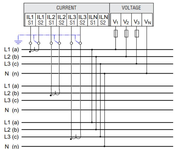
(7) Single-phase measuring, two conductors, without voltage transformers, with one current transformer.
