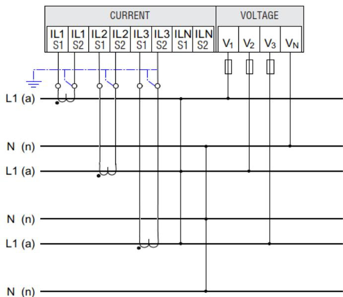
(8) Two-phase measuring, three conductors, unbalanced loads, without voltage transformers with two current transformers.
