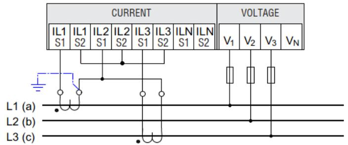
(3) Three-phase measuring, three conductors, unbalanced load, with voltage transformers, with two current transformers. (ARON)
