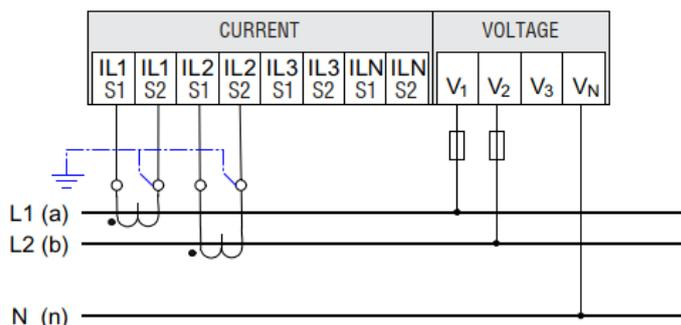
(9) Single-phase measuring, two conductors, with voltage transformers, with three current transformer.
