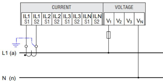
(6) Three-phase measuring, four conductors, balanced multiple loads, with three current transformers.
