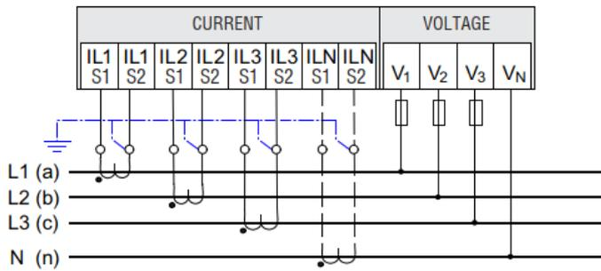
(2) Three-phase measuring, three conductors, unbalanced load, without voltage transformers, with two current transformers. (ARON)
