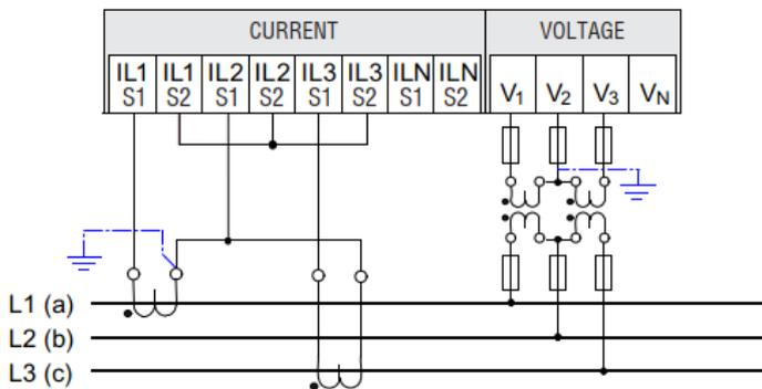
(4) Three-phase measuring, three conductors, balanced load, without voltage transformers, with one current transformer.
