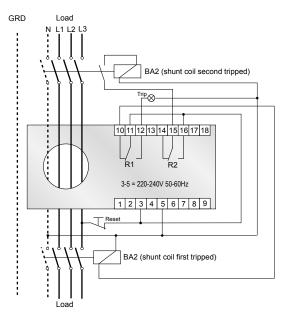
WIRING CONNECTION ELRD-L | ELRD-L2m
